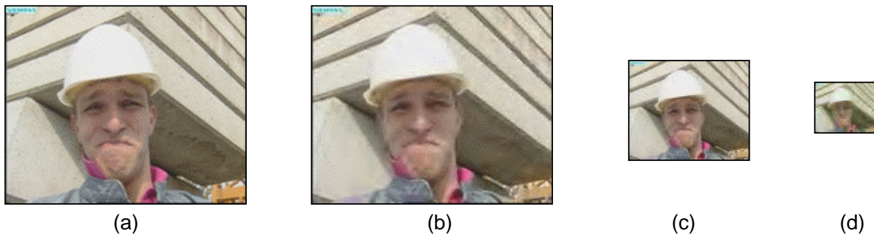
Figure 7: Visual performance comparison with the AnyBandwidth Technology. (a) Original image. (b) Decompressed image at 10 frames/sec, 200 kbps. (c) Decompressed image at 5 frames/sec, 68 kbps. (d) Decompressed image at 2.5 frames/sec, 10 kbps.
